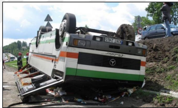
Figure 1.2: Crucial Deformation of Side Pillars.
