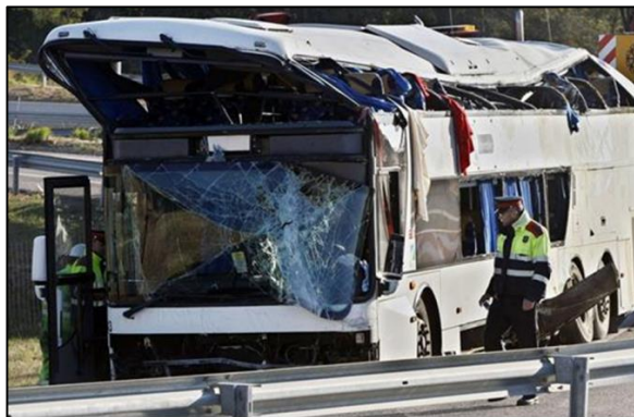
Figure 1.3: Damaged Superstructure of Double-decker Bus.
