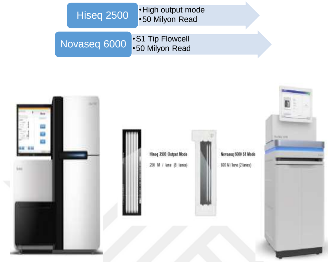
Şekil 3. 20: HiSeq 2500 Output mode ve Novaseq 6000 S1 Mode flowcell.
