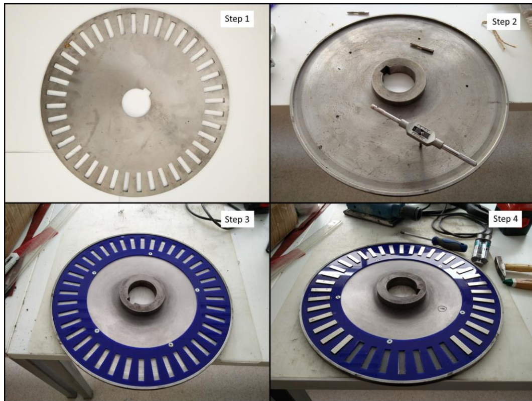
Figure 7.14: Manufacturing of rotors.
