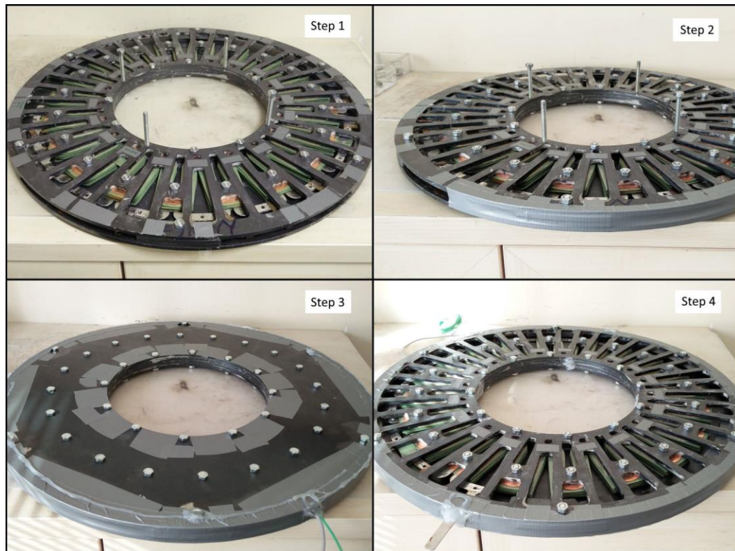
Figure 7.12: Preparation of mold for epoxy casting.
