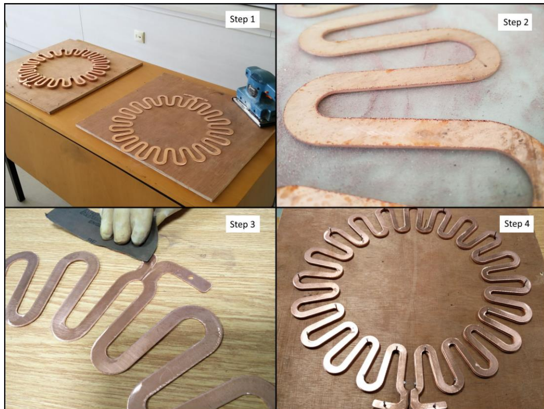
Figure 7.3: Preparing coppers of wave winding.
