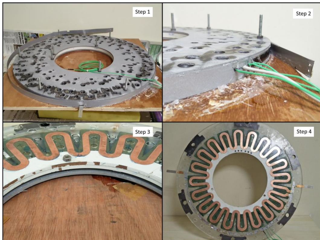
Figure 7.8: Removing process of the stator from the mold.
