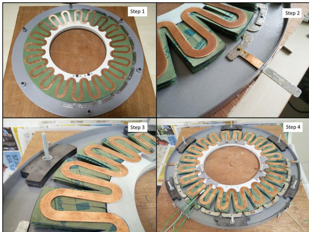
Figure 7.7: Process of arrangement and soldering of windings.
