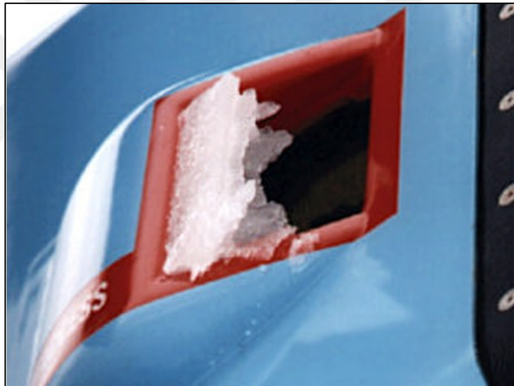
Figure 1.4: EH101 engine bay cooling scoop icing [4].
