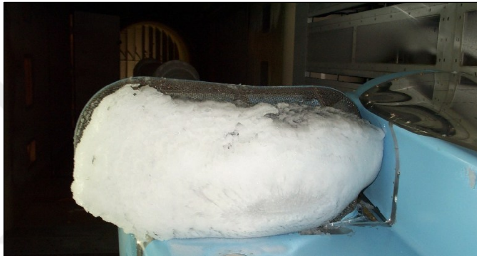
Figure 2.7: NH90 intake icing tests (1200 m altitude, 150 km/h, T=-5^{\circ}\text{C} , \text{LWC}=0.7 ) [16].
