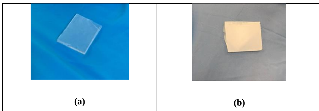
Figure 3.7 The as-spun PVP- \text{TiO}_2 composite nanofibers on glass (a) 5min (b)30min deposition time.
