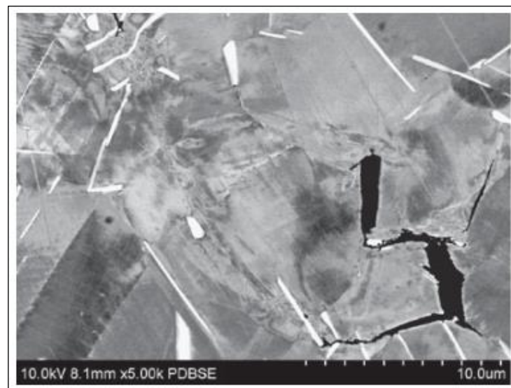
Figure 3.11: Picture of planar slip in the grain surrounding the crack tip at 550 C with 90 s hold time
