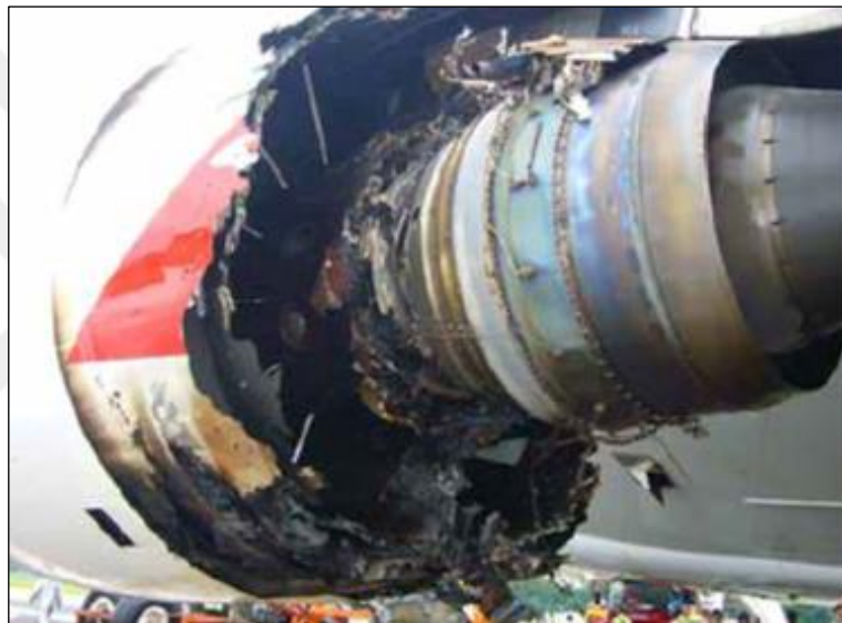
Figure 1.9: Airbus Qantas A380-842-disc burst [10]
