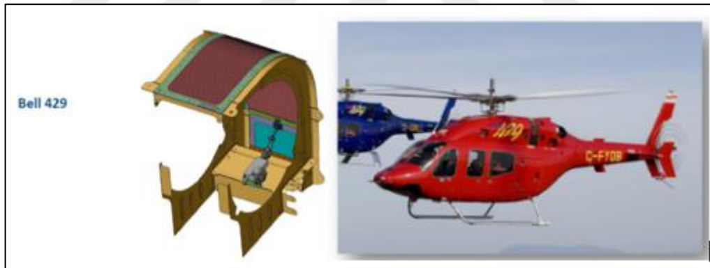
Figure 2.1: Filter integration for Bell 429 platform [10].
