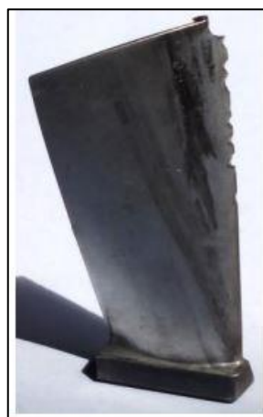
Figure 1.2: Damaged blade by small objects [5].
