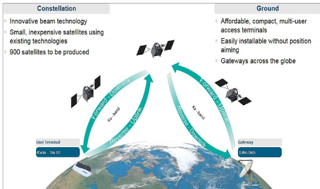
Figure 4.4 : OneWeb communication system overview (image credit:OneWeb)
