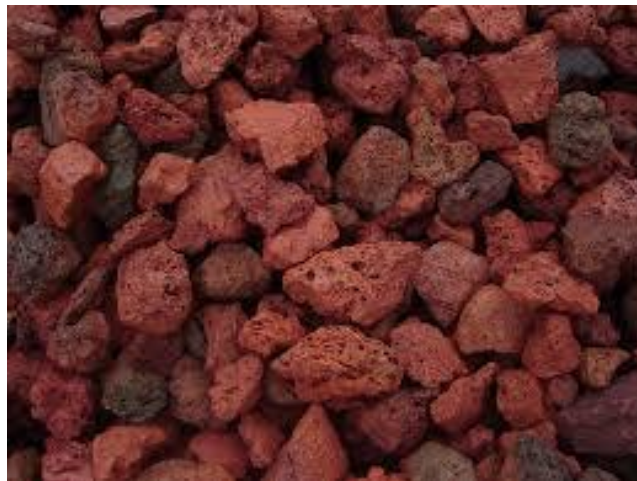
Figure 2.6: Images of Volcanic Slag.
