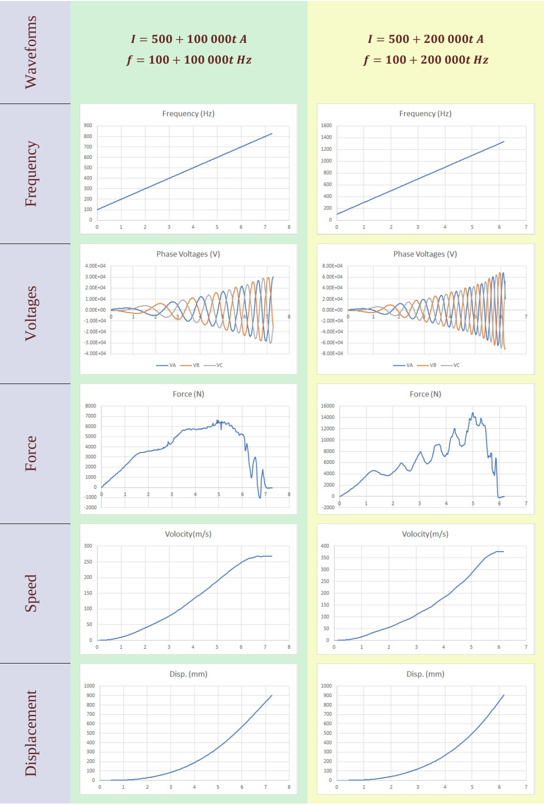
Figure 4.11: The output waveforms under varying current varying frequency values.
