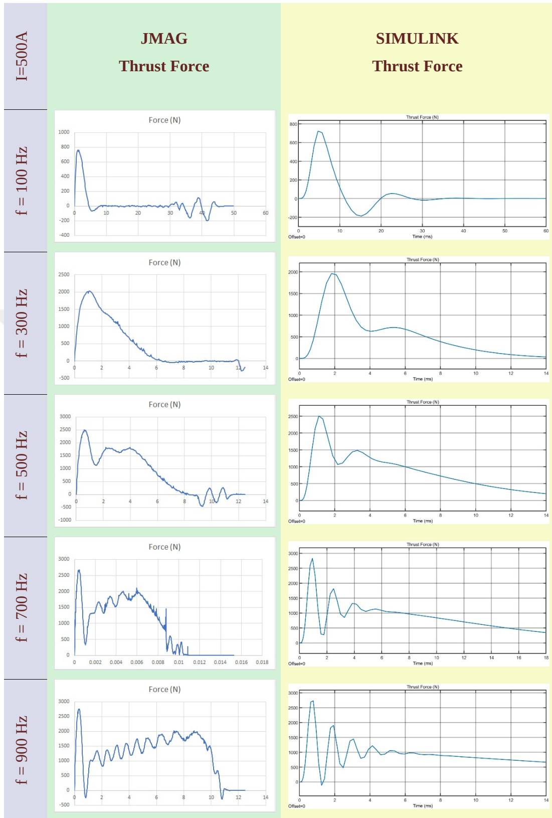
Figure 5.13: Thrust force waveforms, for 500A between 100 Hz and 900 Hz, obtained from JMAG and Simulink model.
