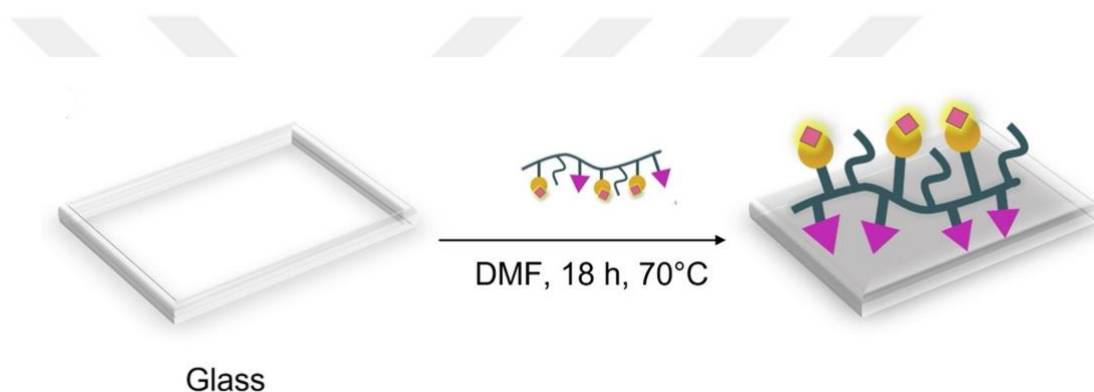
Figure 3.34: Schematic representation of polymeric coatings on glass surface after functionalization of TFBA via epoxy-amine reaction.
