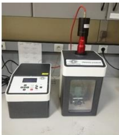
Figure 4.1: Nanao Grafi Ultrasonic Homogenizer [NG-900N] model ultrasonic device used for LPE.
