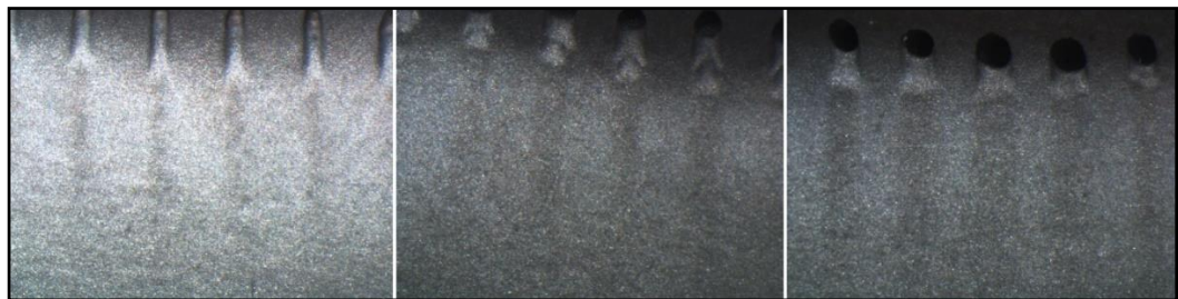
Figure 4.6: Stereo Microscope Images 0,45,90-degree cooling holes.
