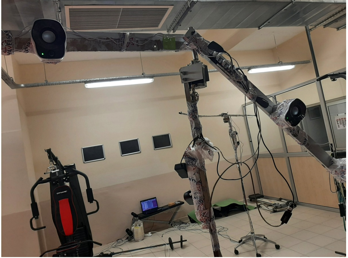
Figure 3.15: The actual RIR data collection system used to collect GTU-RIR dataset.
