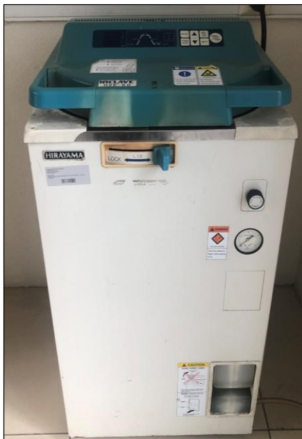
Figure 3.1: Hirayama HVE-50 autoclave device used in the experiments.
