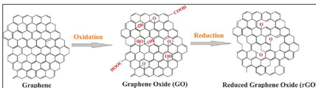
Figure 1.7: Chemical conversion of graphene to GO and rGO [15].
