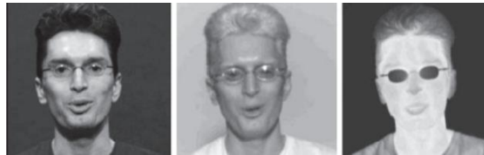
Figure 1.2: A face imaged in the (a) Visible camera, (b) SWIR camera, (c) MWIR camera [2].
