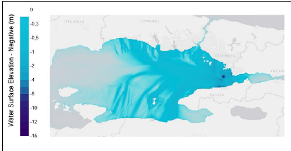
Figure 3.18: The maximum negative water surface elevations calculated in the entire Marmara Sea for Scenario-2 Tuzla landslide.
