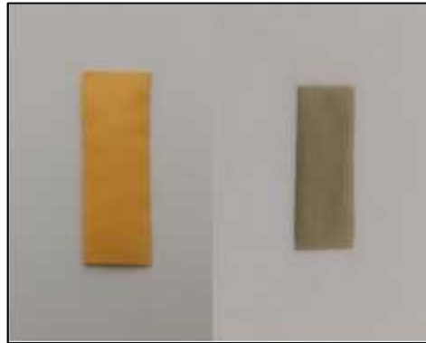
Figure 4.5: Image of the tapes before (left) and after (right) sintering at 1000 °C for 6 hours.
