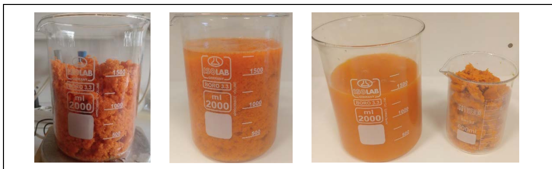
Figure 4.1: Photographs of the processing of carrot medium (CM); defrosted carrot pomace used to make the CM (left), carrot pomace blended with dilute sulfuric acid (middle) and the CM and resulting pomace after the cheesecloth straining (right).
