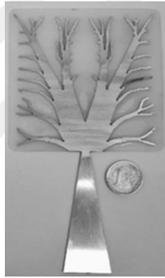
Figure 1. 2: Designed heat sink with topology optimization [2].
