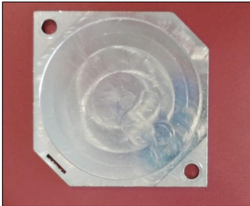
Figure 2.3: Galvanized low carbon steel.
