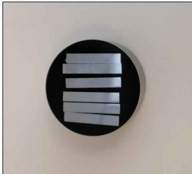
Figure 3.2: Mounted specimens in bakelite resin.
