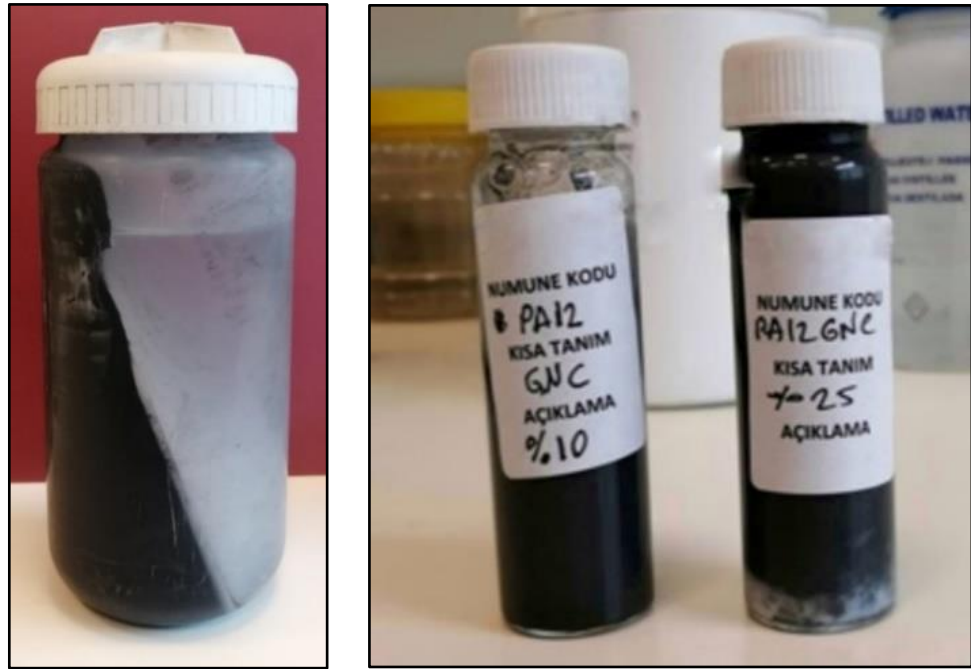
Figure 2.14: a) Separating ethanol from the mixture b) PA12/Water dispersion is prepared.
