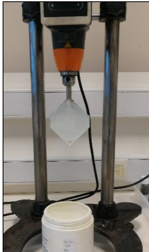
Figure 2.10: The sample coating with a primer.
