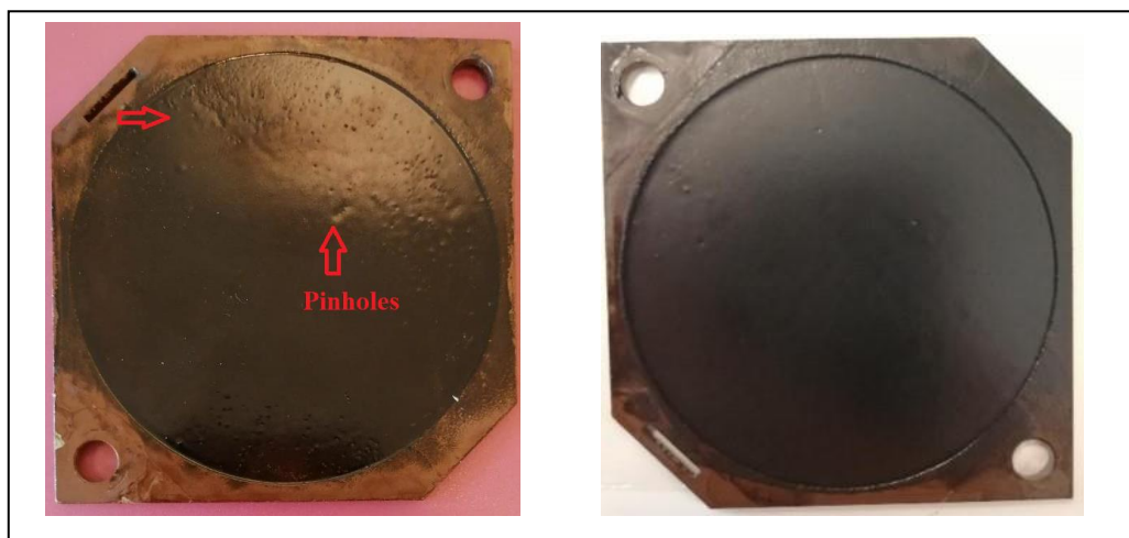
Figure 2.18: a) Single-layer PA12 coating. b) Double-layer of PA12 coating.
