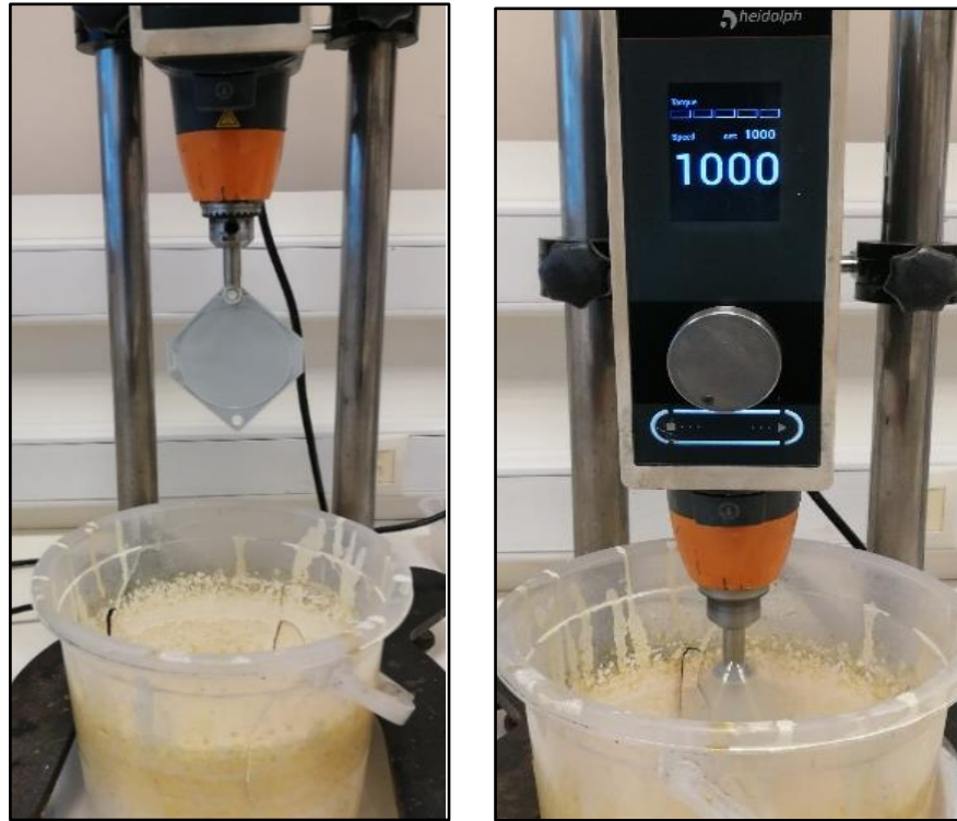
Figure 2.8: a) The sample is removed from granodine b) The sample is rotated at 1000 rpm.
