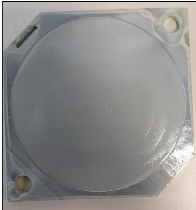
Figure 2.11: Primer and chemical conversion coated low carbon steel.
