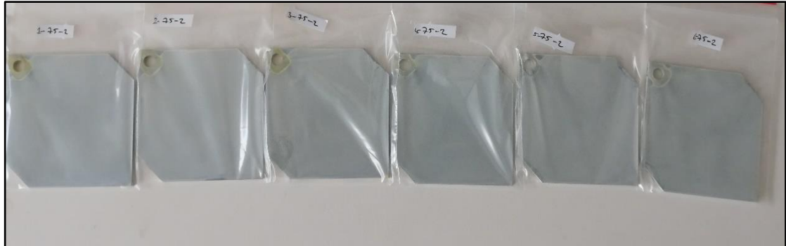
Figure 2.5: The primer-coated samples obtained with 75% primer in the mixture with 2 repetitions.
