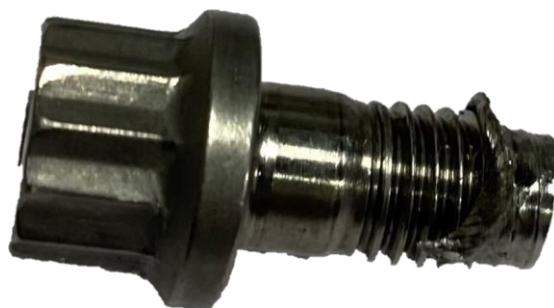
Figure 3.9 Example of a bolt failure during the test.
