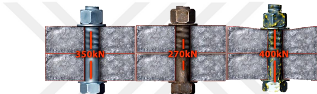
Figure 2.26 Different preload values due to different coefficients of friction under same specified torque [39].
