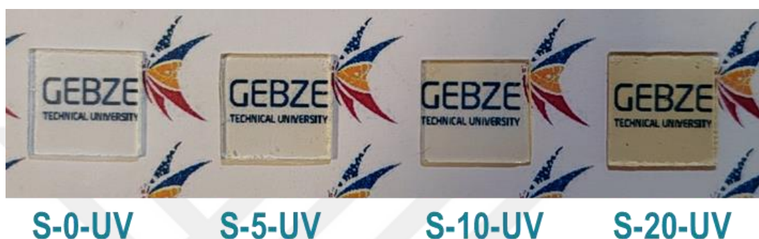
Figure 4.13: Photographs of hydrogel coating on glasses after UV exposure.
