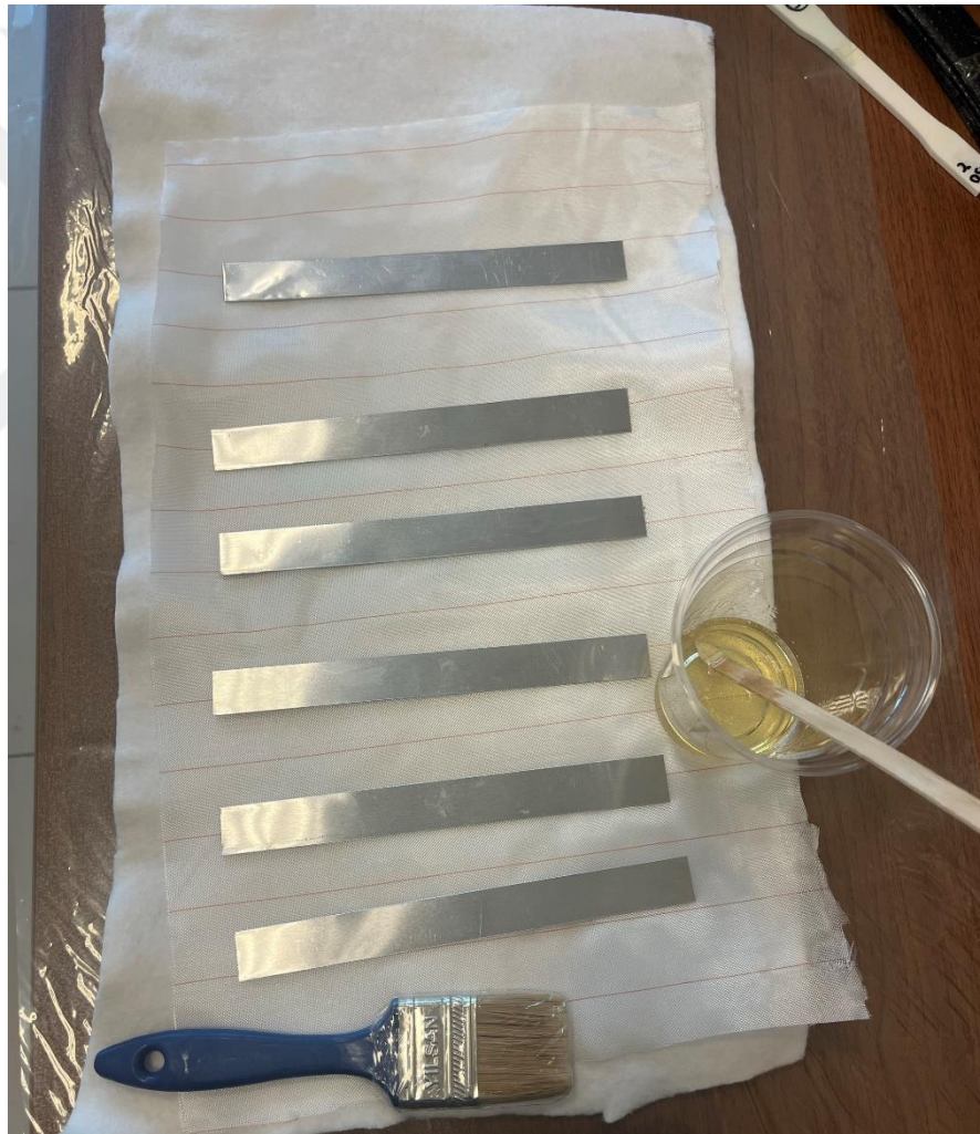
Figure 2.6: Prepared face sheets and bonding process.
