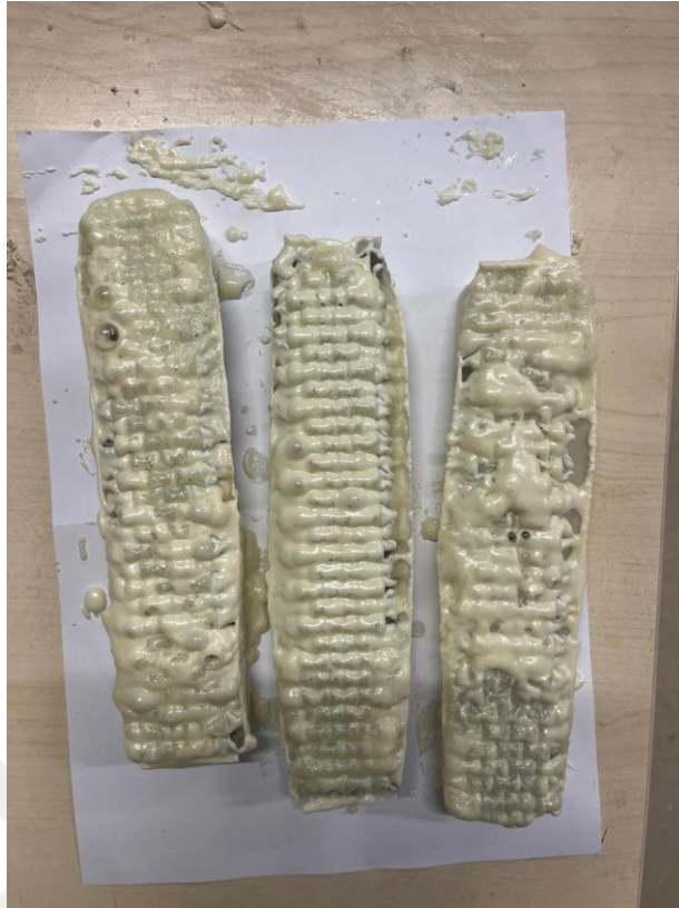
Figure 2.9: Cell voids were filled by pouring foam onto the specimen.
