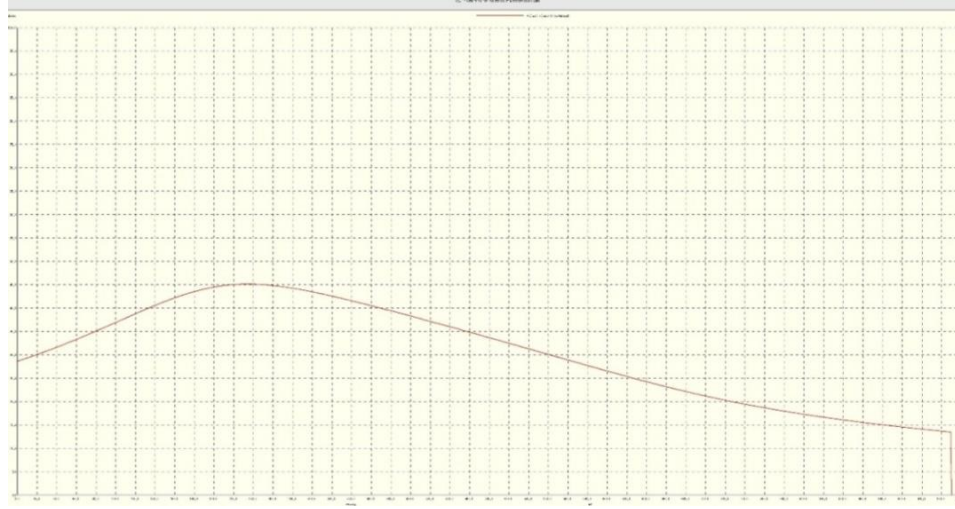
Figure 3.29: Resistance plot of a single transmission gate.
