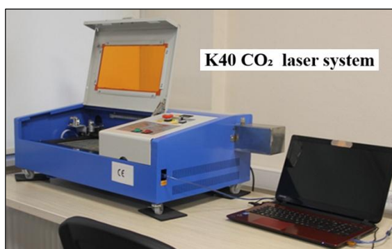
Figure 9.1: Fabrication of laser-induced graphene using a K40 CO 2 laser system.
