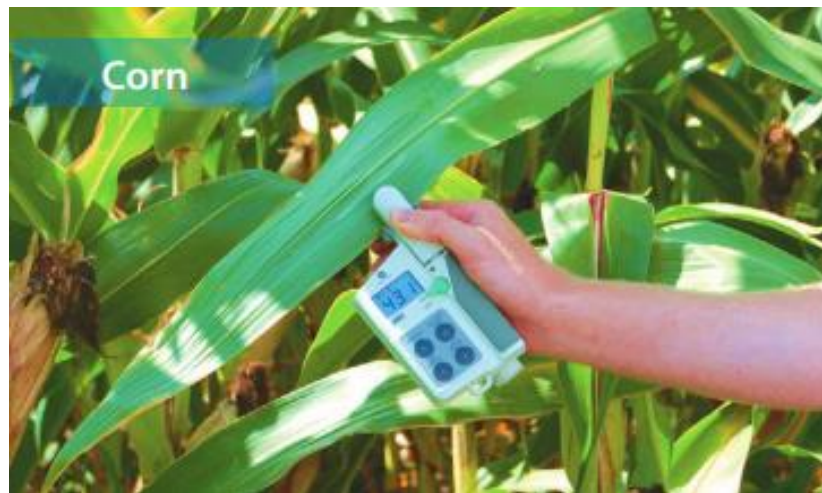
Figure 3.1: Chlorophyll measurement from maize leaf with SPAD-520Plus.
