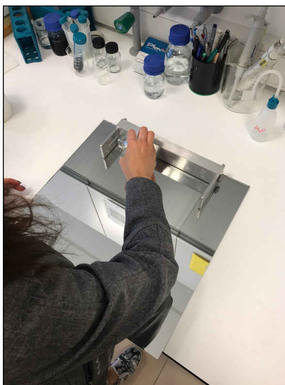
Figure 3.4: Preparation of polysulfone membrane substrate.
