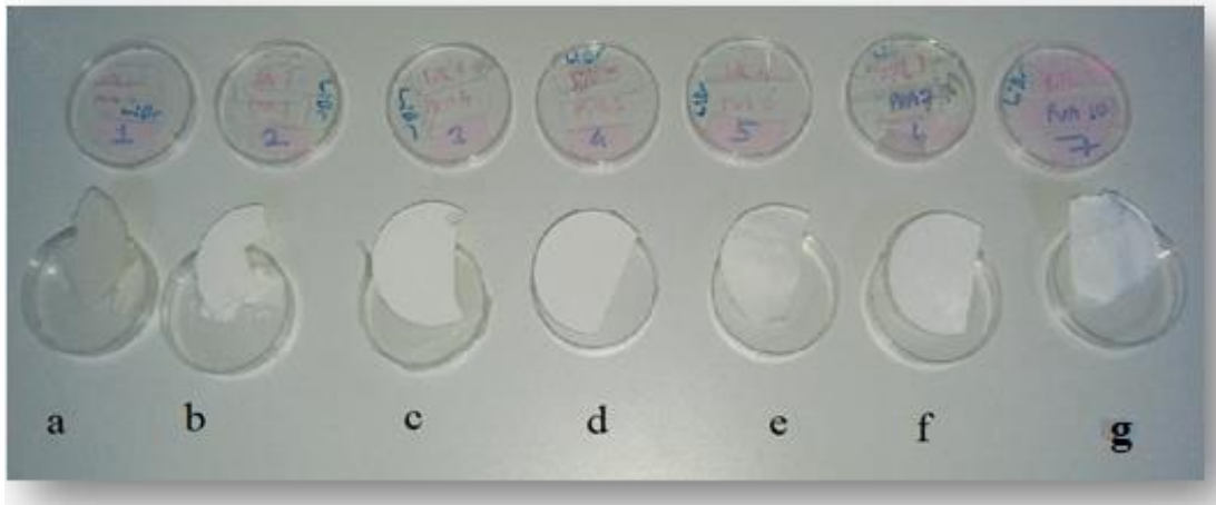
Şekil 3.5: İpek Fibroin (CaCl 2 ) PVA Sünger Kompozit a) PVA/İpek: 0/10, b) PVA/İpek: 3/7, c) PVA/İpek: 4/6, d) PVA/İpek: 5/5, e) PVA/İpek: 6/4, f) PVA/İpek: 7/3, g) PVA/İpek: 10/0.
