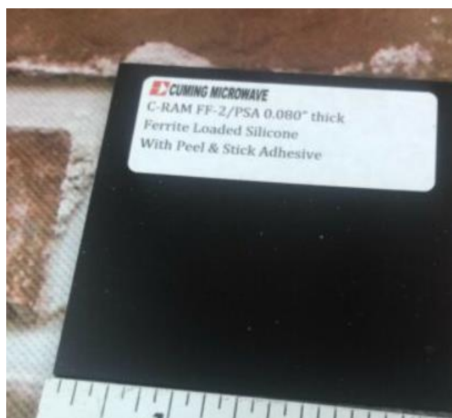
Figure 5.19 Absorber used in PCB case
