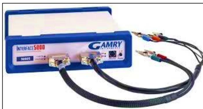
Figure 3.3. GAMRY 5000E Potentiostat.
