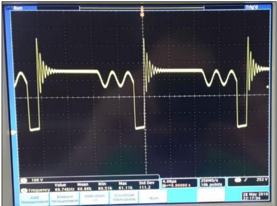
Figure 4.10: Drain-Source Switching Wave Form.
