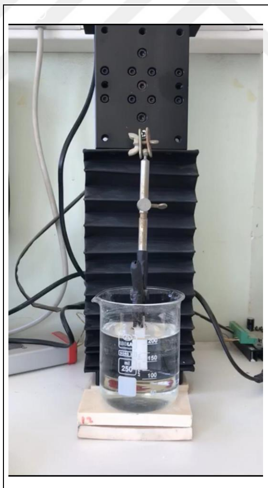
Figure 8.12: Dip-Coating Device and Process
