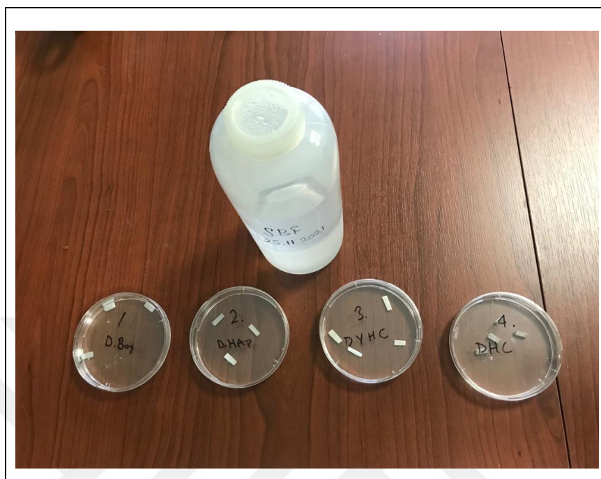
Figure 8.17: Immersion of samples in SBF.
