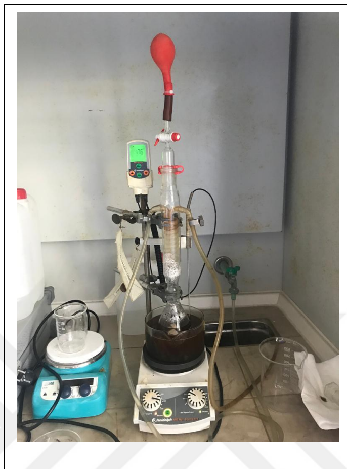
Figure 8.10: Reverse-Flow etching System.
