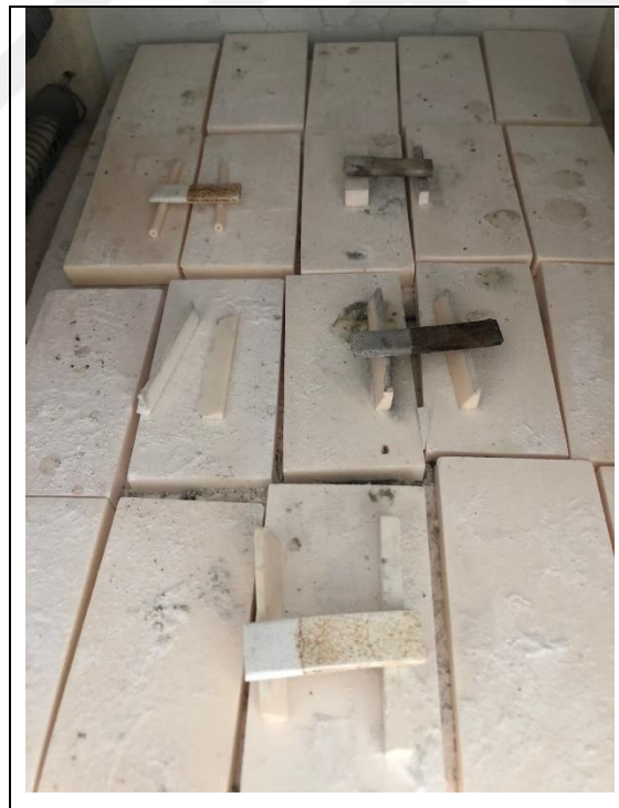
Figure 8.15: Coating before the sintering process with different parameters.
