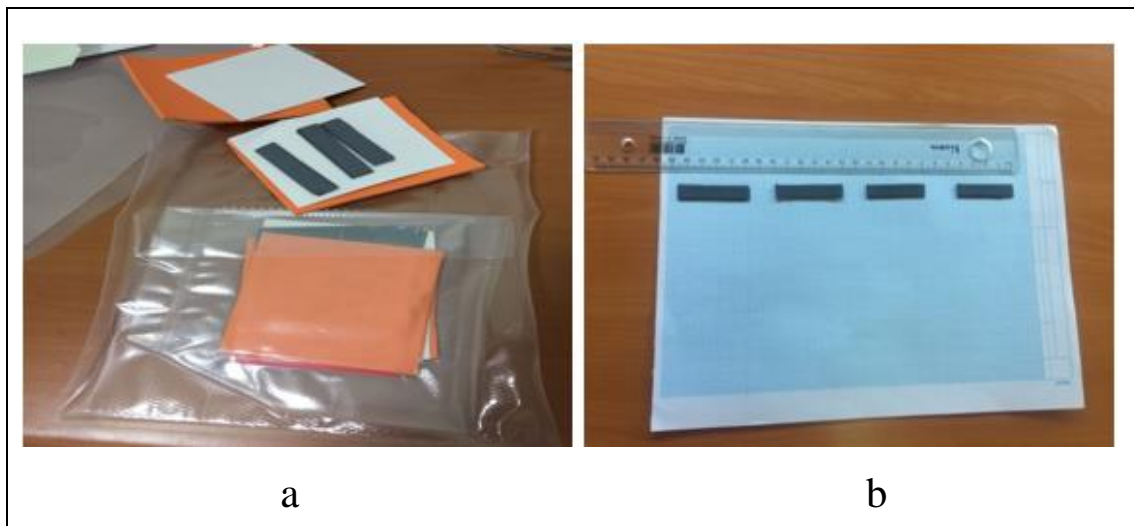
Figure 8.5: a) Preparation for Vacuuming b) After Cold Isostatic Pressing.
