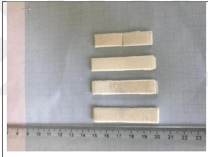
Figure 8.13: Substrates after the coating and calcination.
