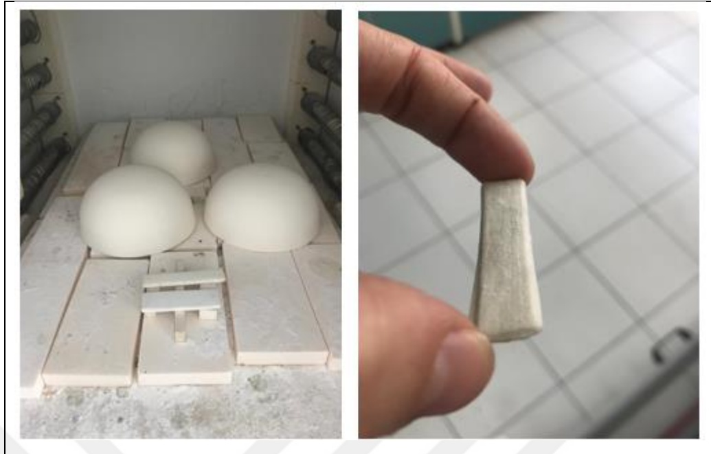
Figure 8.8: Heat treatment process (Left) and final substrate (Right).
