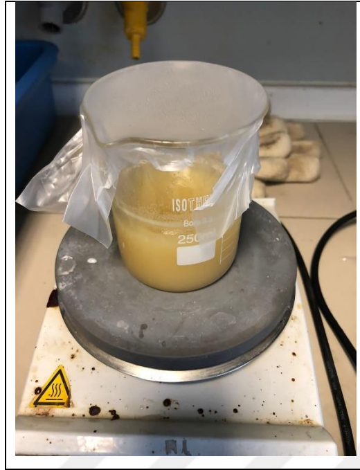
Figure 8.14: Preparation of Chitosan Sols at room temperature.
