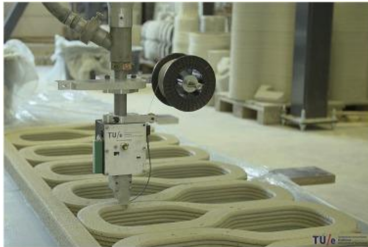
Figure 2.6: Example of 3D Concrete Printing [36]
