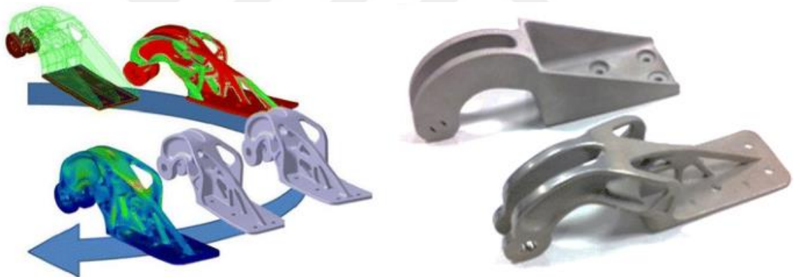
Figure 2.156: : Case study of a topology-optimized bracket [29]
