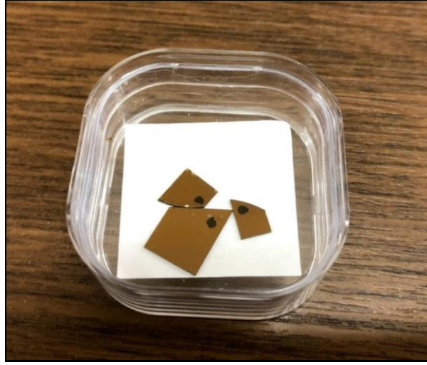
Figure 5.5: Epitaxially grown 5 \mu\text{m} YIG thin films on GGG substrate.
