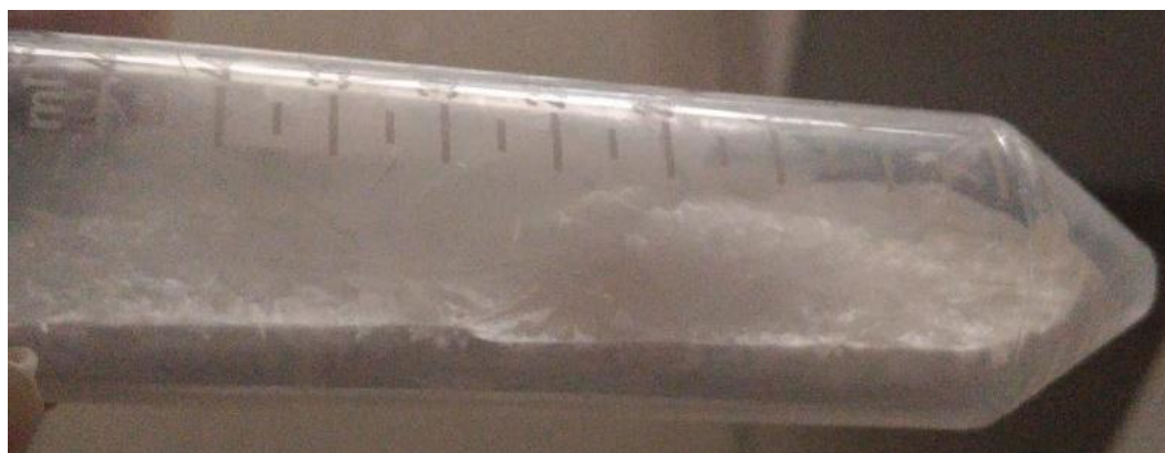
Figure 3.2: Final aspect of GelMA in foam-like structure.
