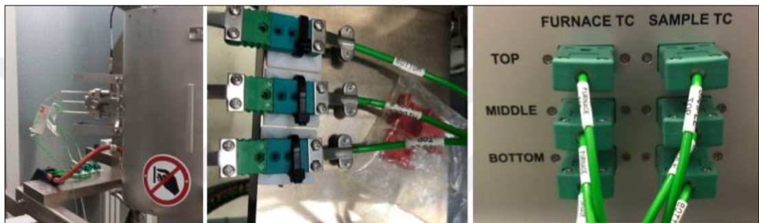
Figure 4.5: Temperature Control Unit Configuration.
