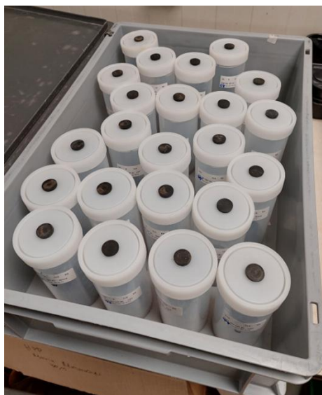
Figure 6.1: 500 mL plastic pots with gas sampling lids used for soil treatments incubation and CO 2 collection.
