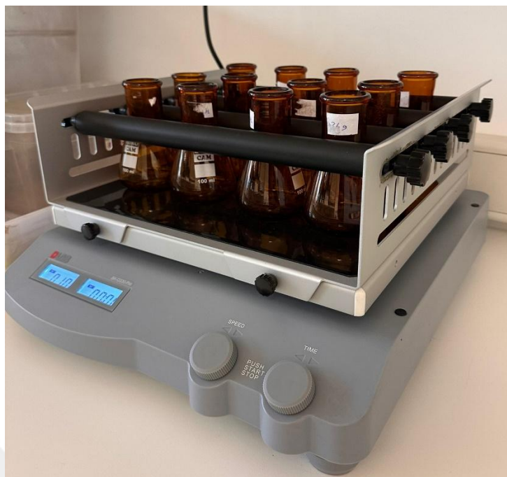
Figure 4.1: The shaker and dark flasks used for the adsorption experiments.
