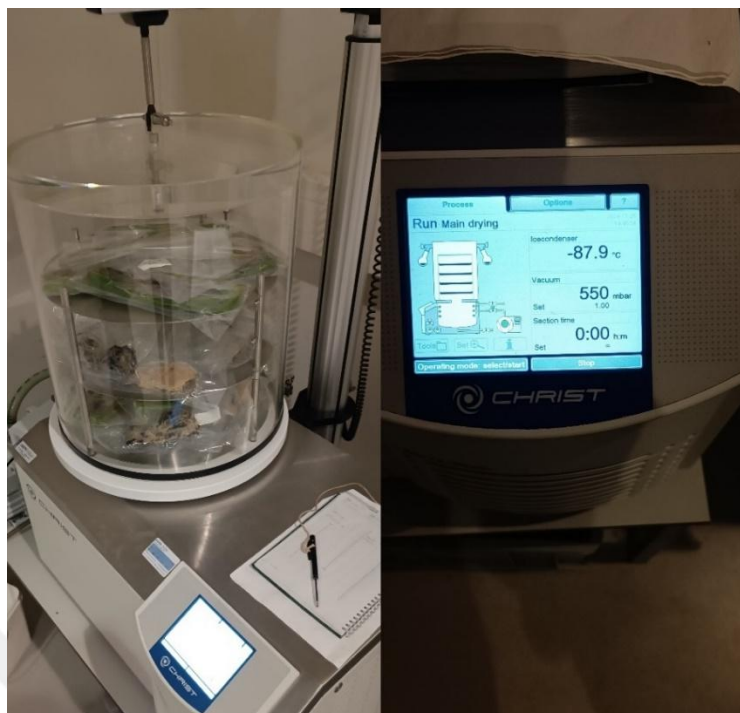
Figure 6.11: The Christ Alpha 1-2 LDplus freeze drier used to dry the harvested maize leaves, shoots and roots.
