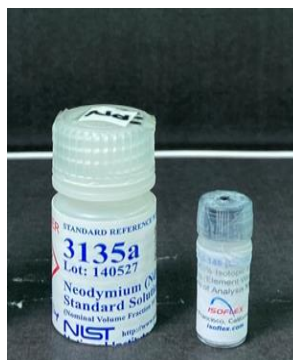
Figure 3.3: NIST CRM 3135a reference material and isotopic RM enriched ^{145}\text{Nd} .
