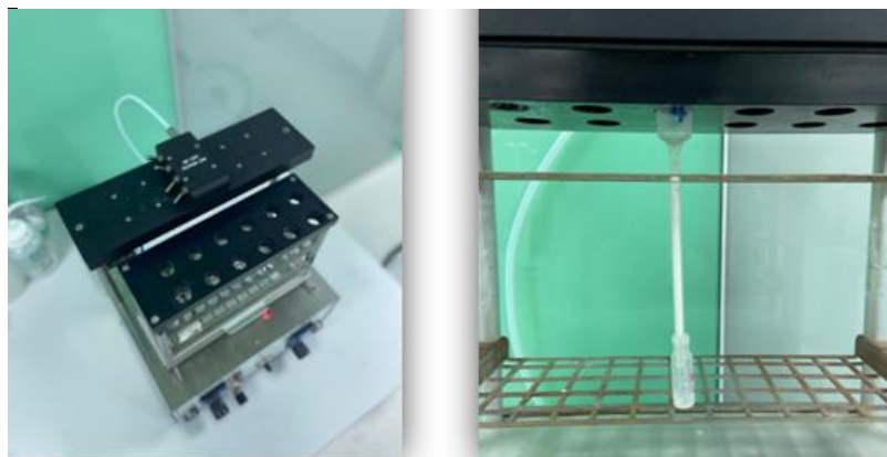
Figure 3.5: Extraction System and PP microcolumn (~ 3 mm i.d. and ~8 cm long).
