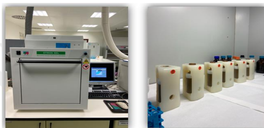
Figure 3.2: Milestone ETHOS SEL with HP 10/1000 rotor.
