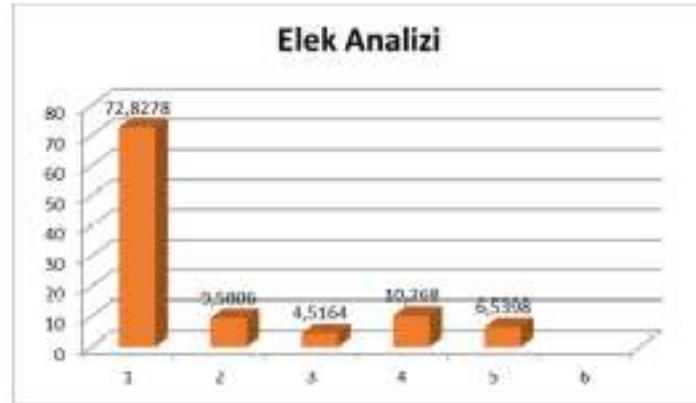
Resim 1: Cam tozu numunesi (<50 µm: 72,8278 gr, 50-63 µm: 9,5806 gr, 63-77 µm: 4,5164 gr, 77-100 µm: 10,368 gr, 100-125 µm: 6,5398 gr).
