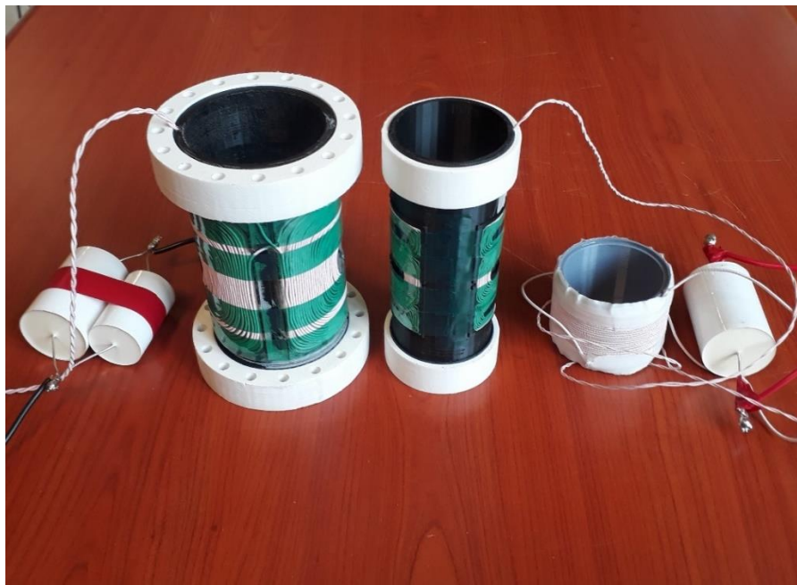
Figure 7.17. Resonance and bandstop filters for drive and receive chain of MPI scanner: (a) Solenoid drive and receive coil system, (b) Saddle drive and receive coil system.
