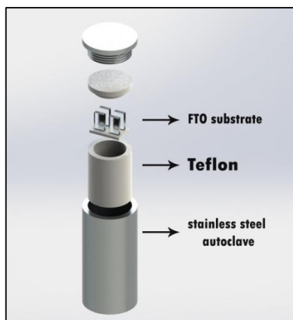
Figure 3.1: Schematic illustration of Teflon and stainless steel autoclave.
