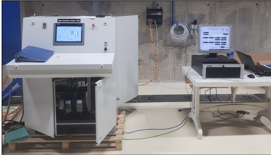
Figure 6.3: Control System and DAS of Fuel System Test Rig
