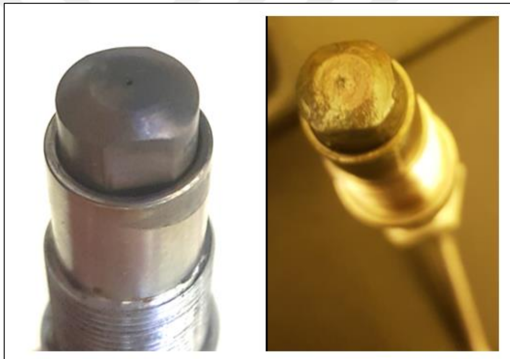
Figure 3.8: Used Pilot Fuel Injectors – Unclogged / Clogged
