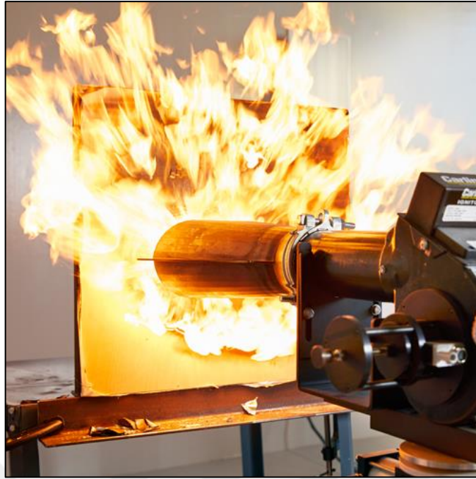
Figure 4.4: Fire Test Burner and Setup
