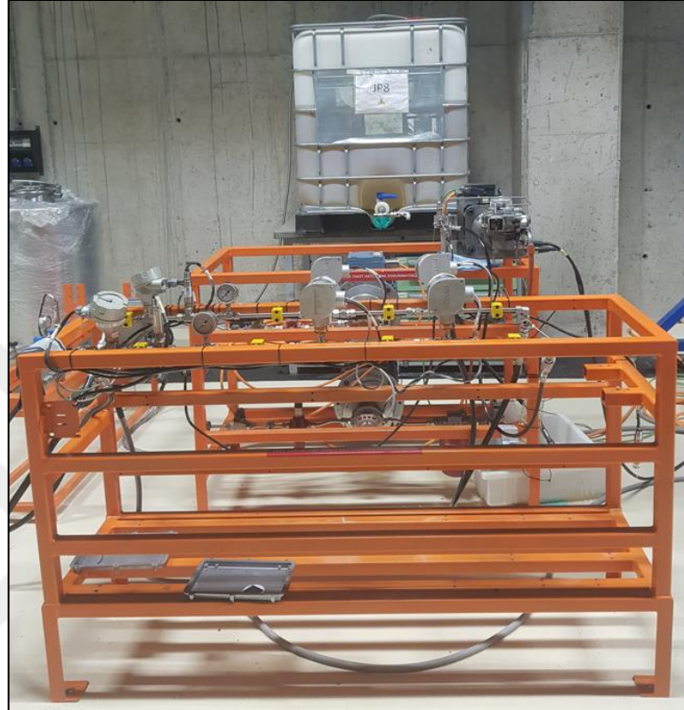
Figure 6.2: Instrumentation Bench Fuel System Test Rig
