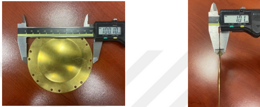
Figure 4.1: Diameter (left) and thickness (right) of the brass end-cap part.
