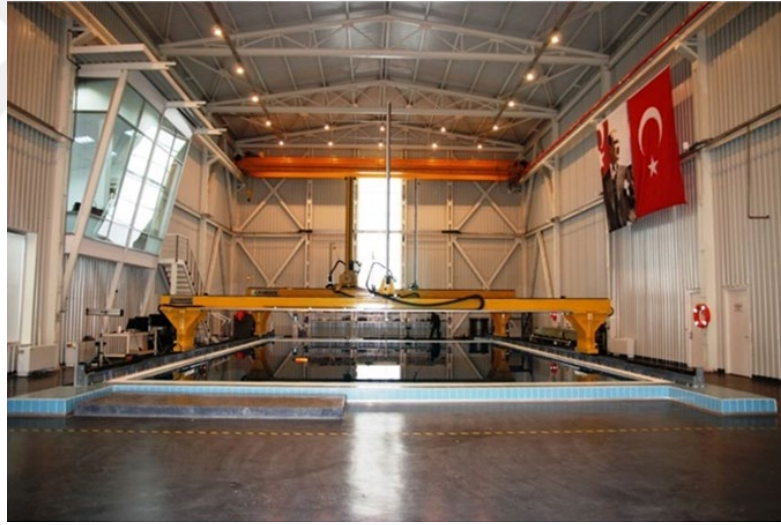
Figure 6.1: The general view of the TÜBİTAK MAM SAL open test tank facility and the Precise Positioning System.
