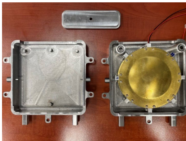
Figure 4.8: The mold structure together with the segmented Class V Flextensional transducer element.
