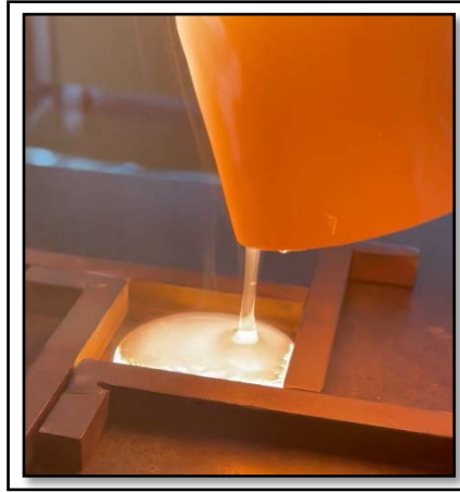
Figure 5.1: Preparation of F1 specimen for CTE measurement.
