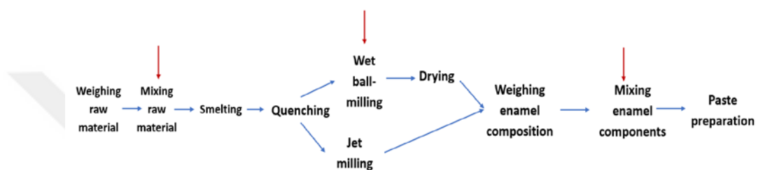
Figure 1.3: Flow chart of production process for glass enamel pastes (blue) and possible addition of carbon reductants (red).
