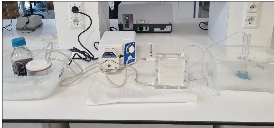
Figure 3.1: Fractionation of unFS and cascade FS products by tangential flow filtration using ultrafiltration units (Vivaflow 200, Sartorius). The sample that could not pass through the cassette and collected in the reservoir (on the left); the sample that passed through the cassette (on the right). (The sample in the reservoir and the sample collected in the filtrate section were kept in an ice box to prevent heating of the samples and cables).
