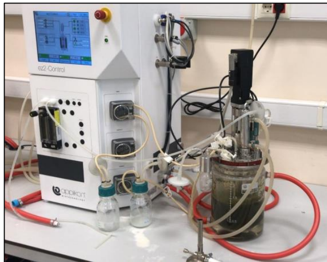
Figure 2.8: A lab-scale stirred bioreactor production set up used in this study.
