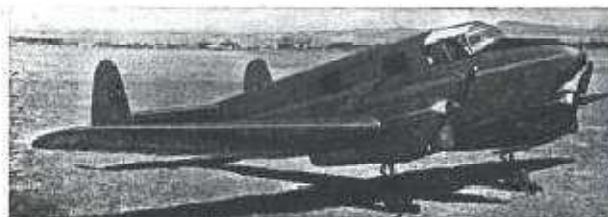
The M.K.E.K. Model 3A Light Transport (two 130 h.p. D.H. Gipsy Major engines).
