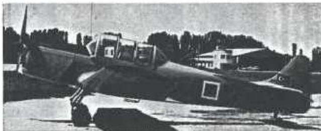
The M.K.E.K. Model 4 Uğur Primary Trainer (145 h.p. Gipsy Major engine).
