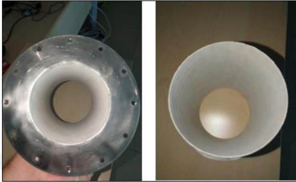
Figure 3.29: Test specimen featuring the applied Thermal Barrier Coating [27].
