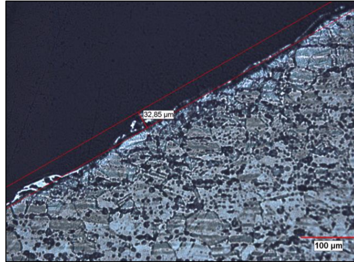
Figure 3.7: Recast Layer Thickness Measurement on Alloy 625 Test Specimen.
