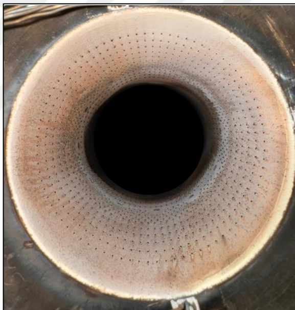
Figure 4.5: Test Specimen After the 750th Cycle – Final Condition.
