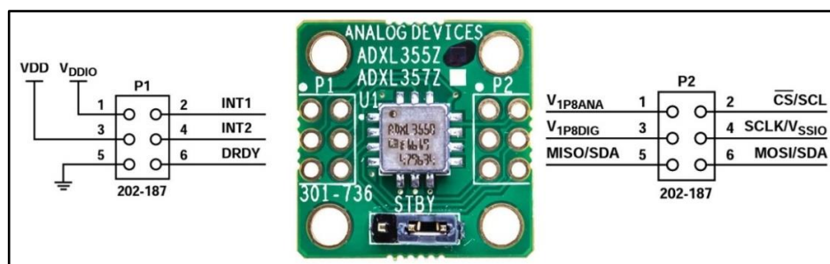
Figure 2.5: CEDAS_acc sensor board header pinout.
